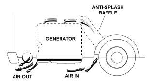
Figure 2.11 – Air Inlet in Vehicle Skirt
